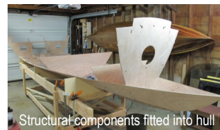
Fitting hull panels to cradle
