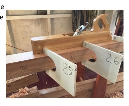
mast was almost 6 inches in diameter at the foot and 2 ¾" at the top where the sheaves assembly was attached. Horizontal lines were drawn for every foot of mast height. Next gauges were made for each foot of height . These gauges would be frequently employed when shaping the mast to the desired thickness at each height.
