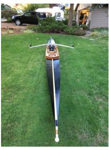
Kavak by Nick Schade, McMillan Press, 1998. Patterns for the bulkheads and bow and stern stem were taken off the full scale sheets from the Wooden Boat Store in Brooklyn, ME. The eight bulkheads and two stems were modified from the originals to fit the rectangular strong back and compensate for the differing skin thickness from the original planned use of 1/8" marine grade plywood to cover the Kingfisher. The strong back is 1-15/16" x 3-15/16", manufactured from 1/2" thick, 4' x 8' cabinet
