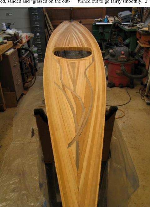
wood all glued together, to form this boat. I glassed and varnished as much of the interior as I could while the boat was still in two halves.
