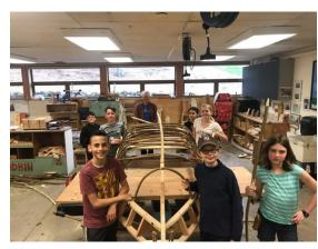
Next the stem and inner keel were made and sandwiched between the gunnels.
