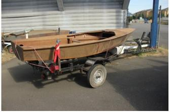
Bouwsma, and Russ Smith, vowed to finish her. Over the course of a year we sanded the hull and deck, removed some filler material which seemed ill chosen, and prepared her for paint. The building plans were with the bag the family gave us so we were able to check what needed to be done. One thing not with her was the centerboard, which we built to the plans and installed. A rudder and tiller was included, so she now had all of her wood. Hardware was another story.
