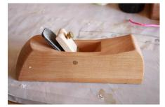
planes, using the plane maker's spruce were glued up to make a first floats made in the previous work- 4" X 4" blank 14' long. This was workshop was shop to fine tune the throats, and then tapered, than marked for 8 building installing the plane irons.
