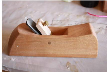
planes, using the plane maker's floats made in the previous workshop to fine tune the throats, and installing the plane irons.
