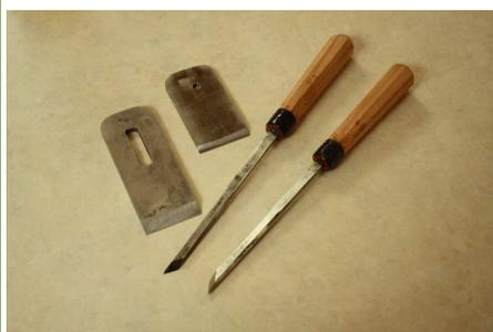
and shaping annealed tool steel maker's floats, marking knives, plane irons, and a set of right and left hand skew chisels. These were then hardened in an oven donated to RiversWest by member Jim Litton, quenched in used cooking oil, and then tempered.
