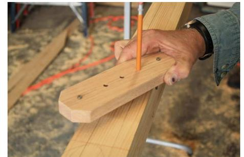
spruce were glued up to make a 4" X 4" blank 14' long. This was then tapered, then marked for 8 sides and power planed, then marked and hand planed to 16 sides, then rounded.
