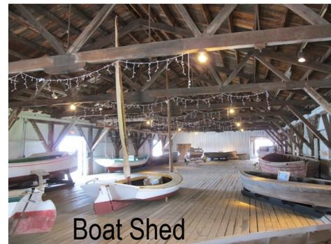
There are several examples of Tilghmann canoes in the shed. These are not canoes as normally thought of, but sailing vessels made of multiple logs shaped in the dugout method. Multiple pine logs were pinned
