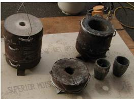
forges were built to Sam's specifications. Bronze casting has been around for thousands of years and can be done with primitive equipment, which is one of the big attractions. Refractory cement is used to build the furnace using a sawn up 5 gallon can, creating a base, a lid, and a cylindrical furnace with a hole in the side to insert a pipe. The pipe is attached to a propane tank, and a small blower is used to inject oxygen. The temperature of the molten metal is 2300 degrees Fahrenheit.
